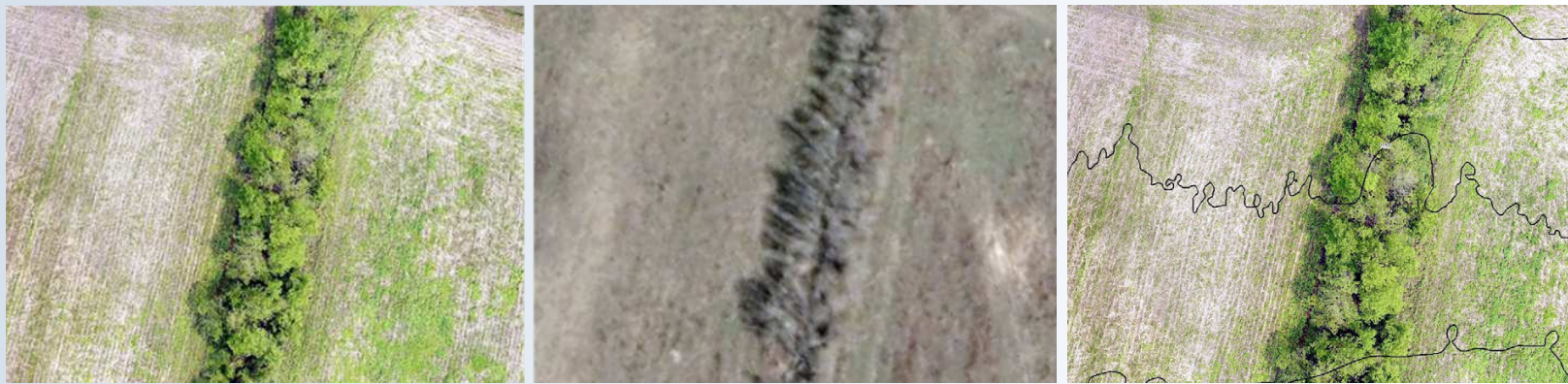
Above left: June 5 Drone flight: 0.9" resolution, Above center: 2017 NYS DOQQ 1' resolution, Above right: Same area with interpolated 2' contours (contours can be exported at any resolution). Areas with tree canopy are filtered out automatically by the software, leaving bare earth data, but if the canopy is too thick, the true ground elevation is not captured and would require supplemental survey points for accuracy. It would be interesting to do a similar flight earlier in spring to see if leaf-off conditions would allow the software to read the ground elevation through brush.
