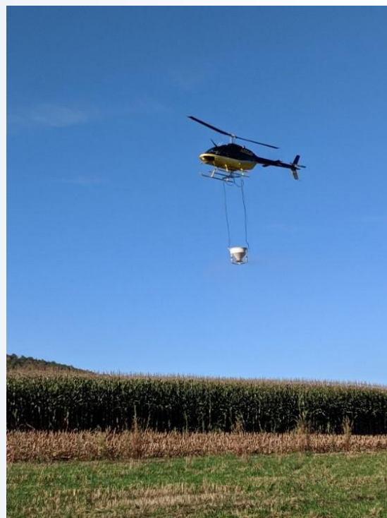
The pilot flew the helicopter approximately 50 ft high in a precise, GPS guided pattern over the cornfield to ensure that all areas were evenly covered.
